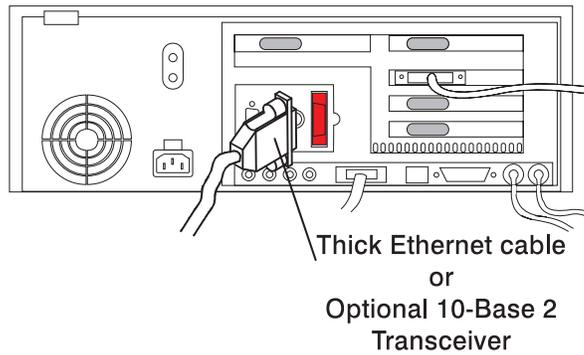
2. Lock the thick cable to the Ethernet connector by sliding the Ethernet connector toward the large notch.
